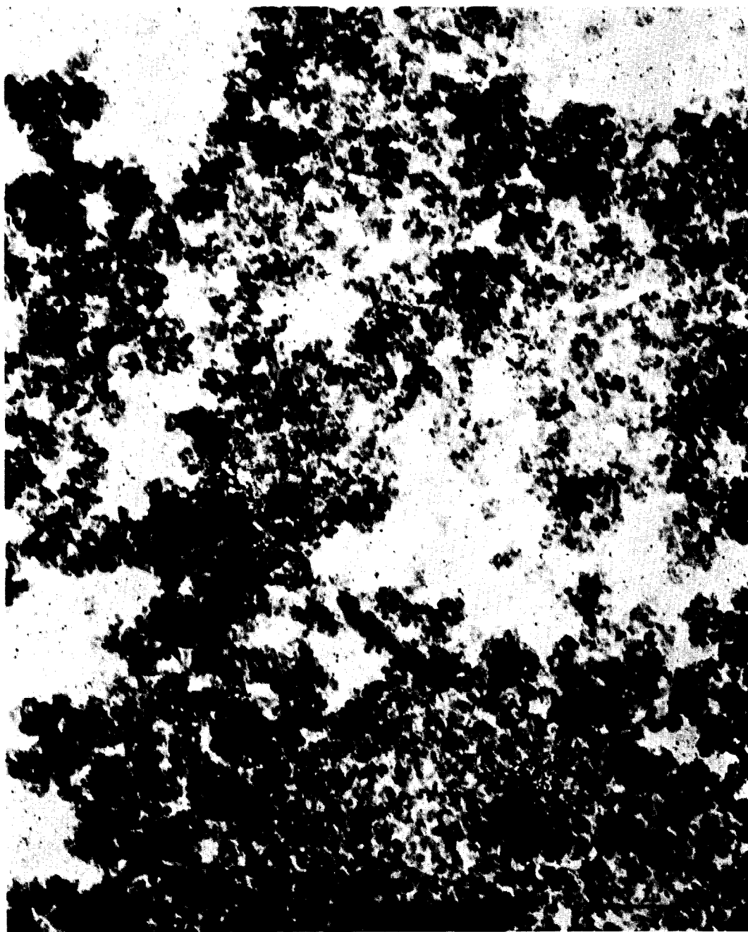
FIG. 1. 2.5% Pt on silica gel, reduced at 210°C. 150,000 \times .
